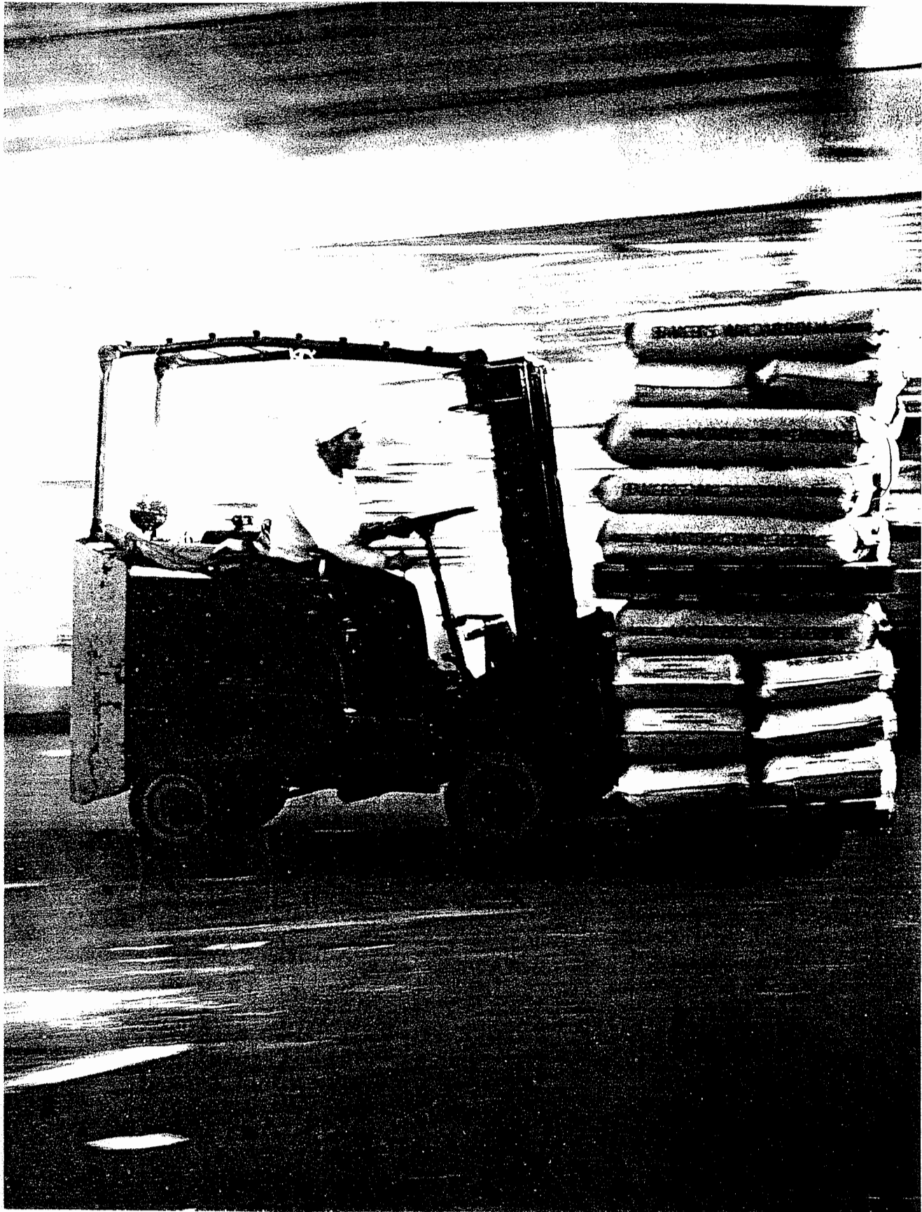
This fork-lift, moving two pallet board loads at a time, is high-piling on the dock.
